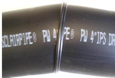
**Figure 9** - Pipe angled in the fusing unit
