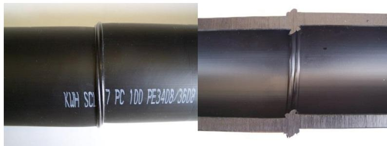
**Figure 7** - Pipe misalignment (high-low misalignment)
