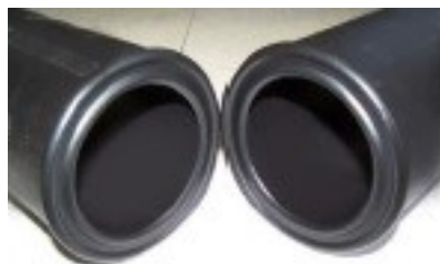
Figure 2 - Unacceptable Concave Melt Appearance
