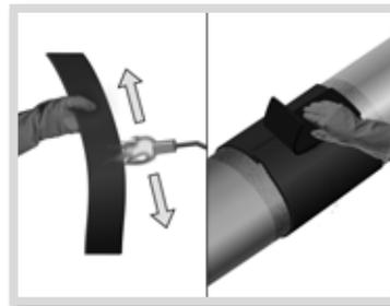
Step 11: Heat the adhesive side of the closure to activate the adhesive before centering the closure over the overlap and pressing it firmly down into place
