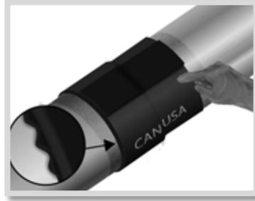
Step 17: After shrinking, press down on the sleeve to ensure adhesive flow over the entire surface. Special attention should be given along the circumference between 4 and 8 o'clock and along the overlap area. In order to avoid a channel formation at the step down, the sleeve should be pressed down. The shrinking has been completed when an adhesive ooze begins at the sleeve edges all around the circumference.
