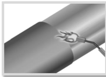
Step 5: Dry the surface of the casing and jacket pipe (width of sleeve + 2" on each side) with moderate flame intensity. Clean the surface with a dry, grease and lint-free rag to remove any grease or dirt.
