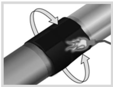
Step 13: Using the appropriate torch, begin at the centre of the sleeve and heat circumferentially around the pipe. Use broad strokes. If utilizing two torches, operators should work on opposite sides of pipe.
