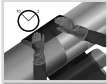
Step 8: Centre the sleeve over the area to be sealed, so that the sleeve overlaps between the 10 and 2 o'clock positions. Press the underlap firmly into place.
