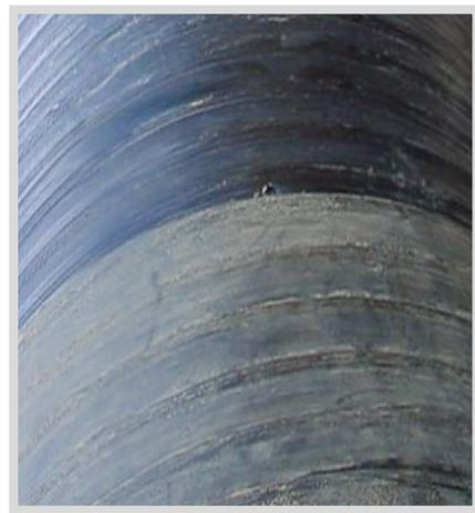
Step 4: Visually inspect the joint to ensure that male and female threads are engaged.
