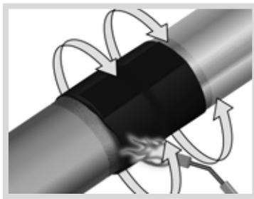
Step 14: Continue heating from the centre toward one end of the sleeve until recovery is complete. In a similar manner, heat and shrink the remaining side.
