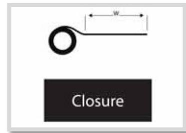
Step 3: Cut the required length (W) of sleeve material from the bulk roll. To ensure that the closure is ready for installation, make sure that there is no dirt or moisture on the closure and that the closure is not damaged.
