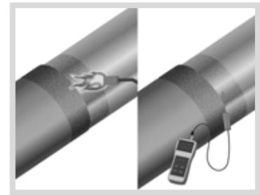
Step 6: Using medium to high intensity flame, pre-heat and activate the surface to be covered with heat shrink sleeve and min 2" on each side of the sleeve to a minimum temperature of 150°F. The flame shall be kept perpendicular to the surface of the pipe and casing during preheating. Check the temperature around entire circumference of the pipe with a touch probe.
