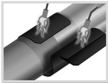
Step 10: Wrap the sleeve loosely around the pipe, ensuring the appropriate overlap. Gently heat the backing of the underlap and then gently heat the adhesive side of the overlap.
