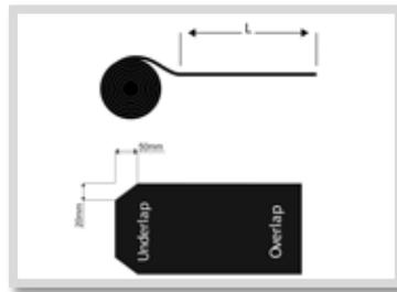
Step 2: Cut the required length (L) of sleeve material from the bulk roll. To ensure that the sleeve is ready for installation, make sure that there is no dirt or moisture on the sleeve and that the sleeve is not damaged.
