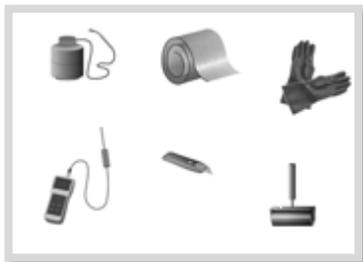
Step 4: Propane tank, hose, torch & regulator, knife, roller, digital thermometer with suitable probe and standard safety equipment; gloves, goggles, hard hat, etc.
