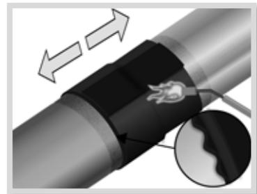
Step 15: Shrinking has been completed when the adhesive begins to ooze at the sleeve edges all around the circumference of the pipe. Make sure the edges of the sleeve are not lifting anywhere around the circumference of the pipe. Finish shrinking the sleeve with long horizontal strokes over the entire surface to ensure a uniform bond.
