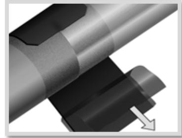
Step 9: Remove the remaining release liner.
