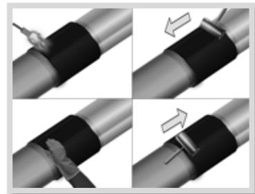
Step 12: Heat the closure with a moderate flame intensity and pat it down with a gloved hand or a roller across its entire length. Make sure that the closure is firmly attached to the underlying sleeve and it is not lifting anywhere. Smooth any wrinkles by gently working them outward from the center of the closure with a roller or by patting the closure down.
