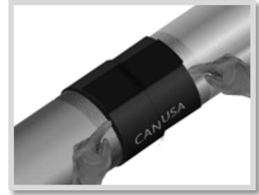
Step 18: As a final check, ensure that the sleeve follows the entire contour of the surface and that there are no cold spots or burning of the sleeve. Make sure the edges of the sleeve are not lifting anywhere around the circumference of the pipe. This can be checked by feeling the edges all around the circumference of the sleeve. If there is edge lifting, the edge should be reworked with additional heat.
