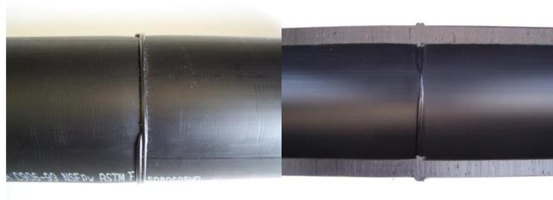
**Figure 8** - Incomplete facing or insufficient heat time
