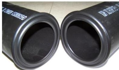
**Figure 2** - Unacceptable Concave Melt Appearance
