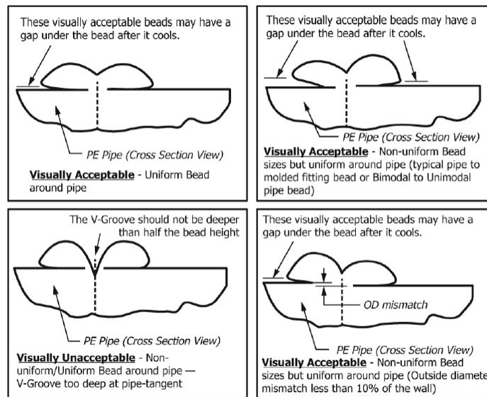
**Figure 3** – Outside Diameter Butt Fusion Bead Guideline as per ASTM F2620
