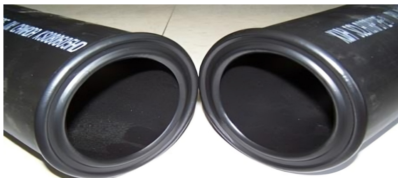
Figure 2 - Unacceptable Concave Melt Appearance
