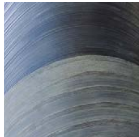
Step 4: Visually inspect the joint to ensure that male and female threads are engaged.
