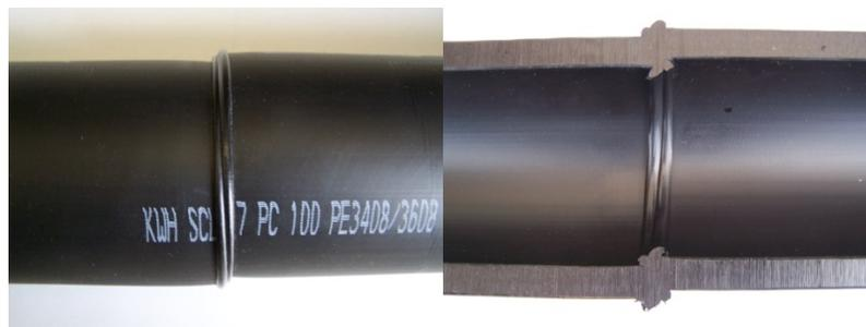
**Figure 7** - Pipe misalignment (high-low misalignment)
