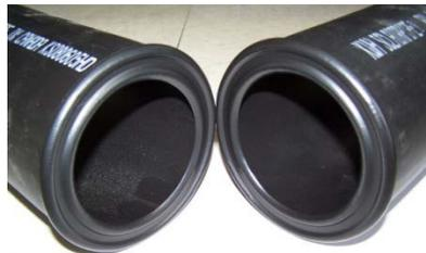
**Figure 2** - Unacceptable Concave Melt Appearance
