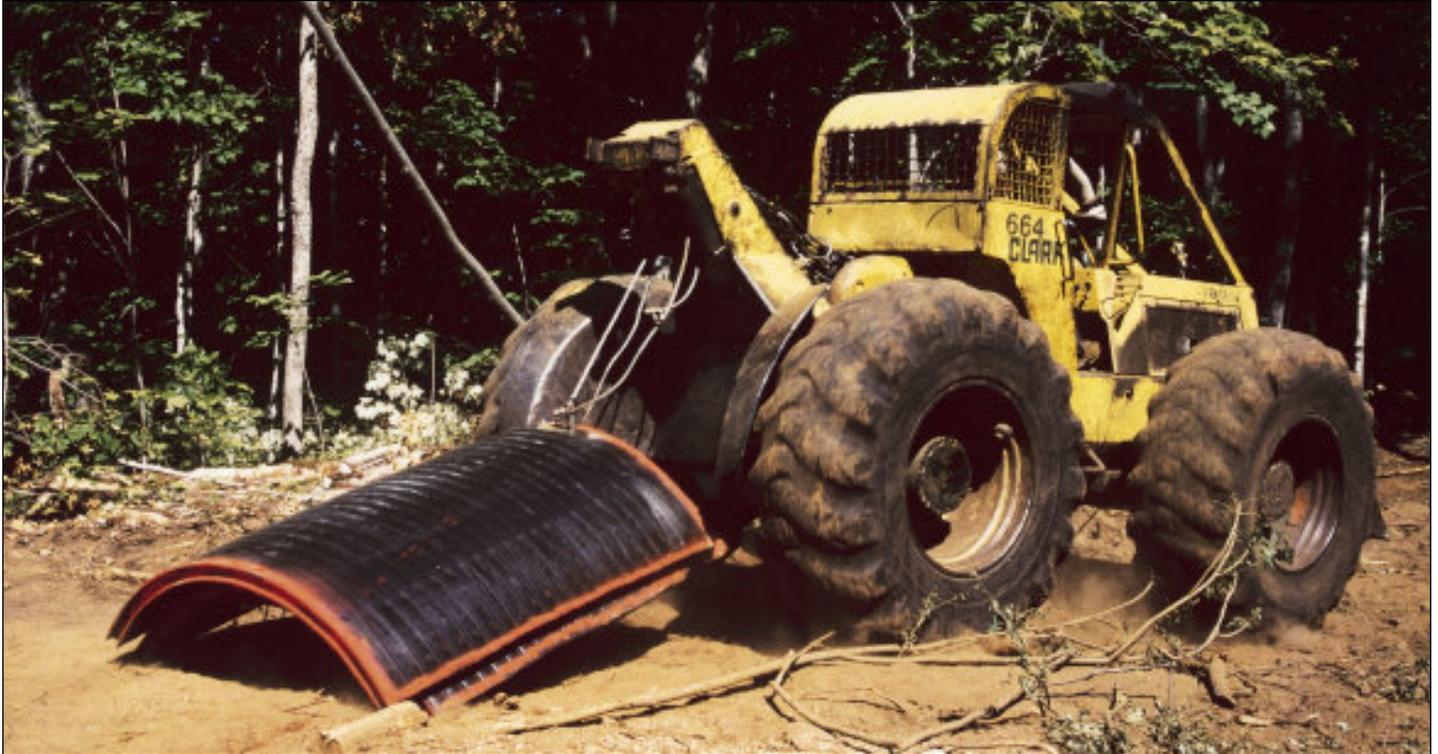
**Project:** Arch Culvert for Logging Operations
